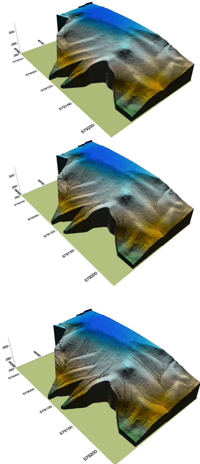
**FIGURE 13** East waste rock dump at 10 (top), 50 (middle) and 100 years (bottom) using postorganic mat parameters. [Color figure can be viewed at [wileyonlinelibrary.com](http://wileyonlinelibrary.com)]
