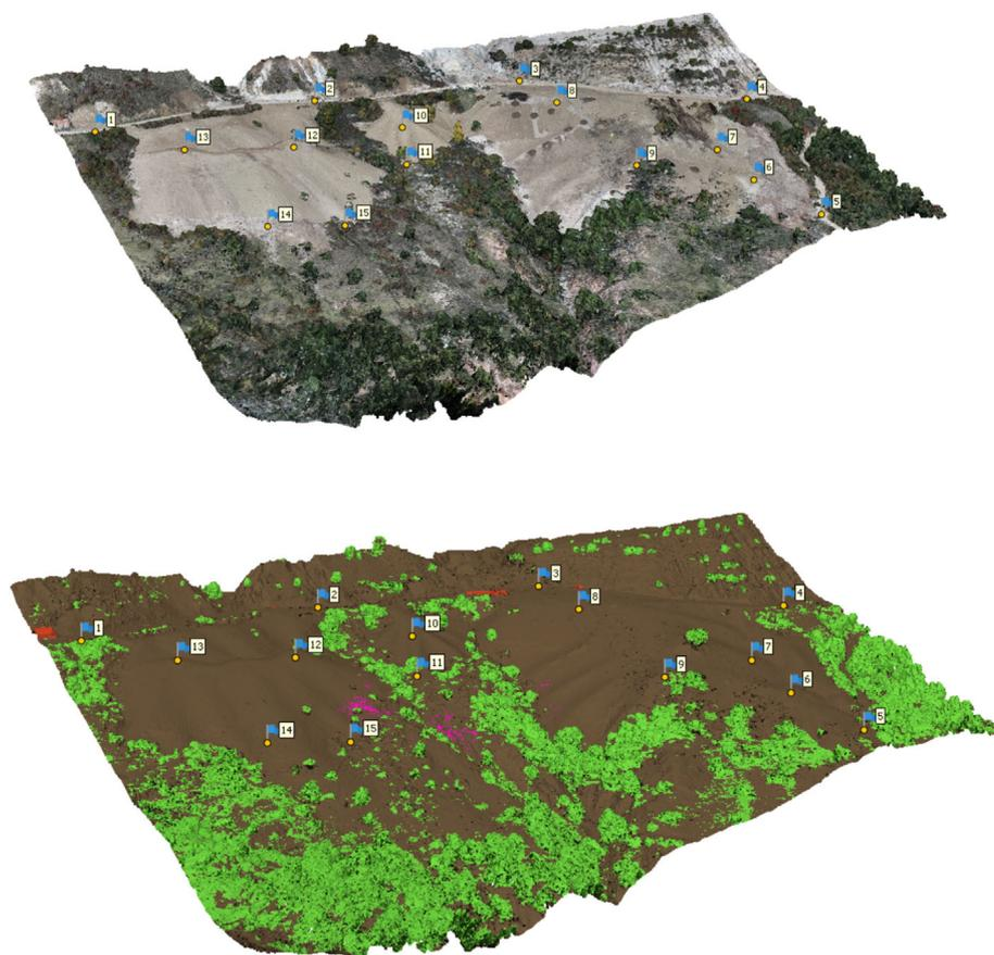
**FIGURE 6** View of the dense point cloud for the external waste dumps, classified (brown, ground; green vegetation; pink, noise) for the reconstructed hillslopes. [Color figure can be viewed at [wileyonlinelibrary.com](http://wileyonlinelibrary.com)]
