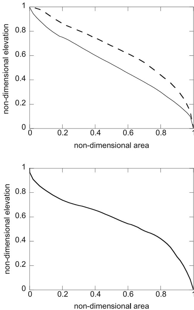
**FIGURE 8** Hypsometric curves for EWRD (top) and WWRD (bottom) geomorphically reconstructed landscapes. Due to the complexity of the EWRD, the landscape hypsometric curves were determined for the two largest subcatchments hence the solid and dotted lines. The curves represent landscapes that are at or near a mature form similar to catchments that have evolved via natural fluvial processes rather than being constructed as in this study. EWRD, East Waste Rock Dump; WWRD, West Waste Rock Dump.
