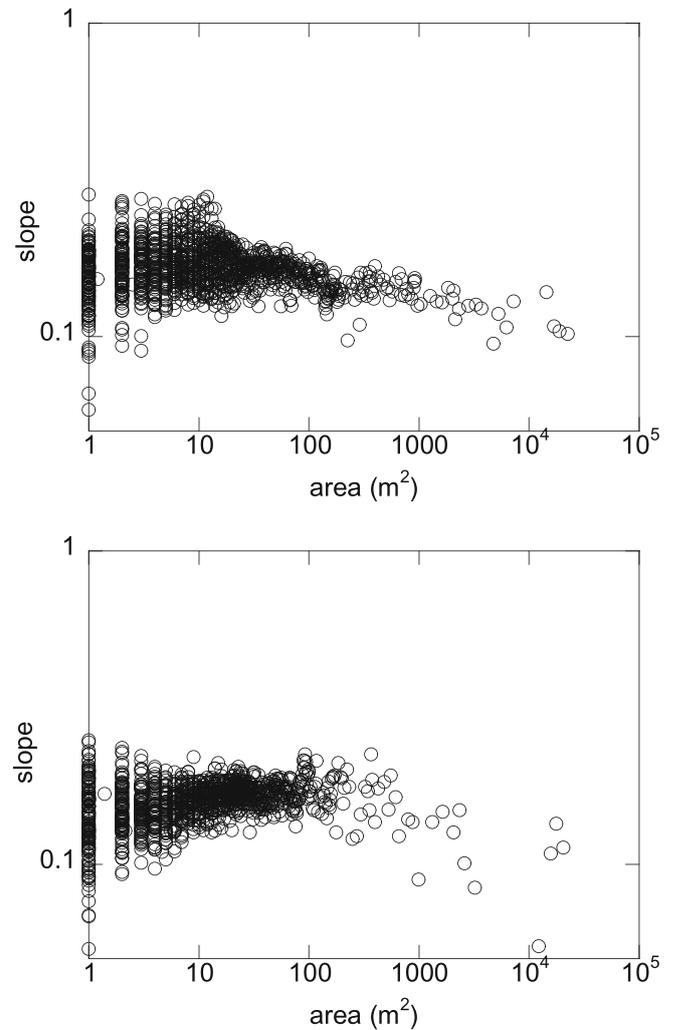
**FIGURE 9** Area-slope relationship for EWRD (top) and WWRD (bottom) geomorphically reconstructed landscapes. The data represents landscapes which have evolved via similar diffusive and fluvial processes as that of natural processes. EWRD, East Waste Rock Dump; WWRD, West Waste Rock Dump.
