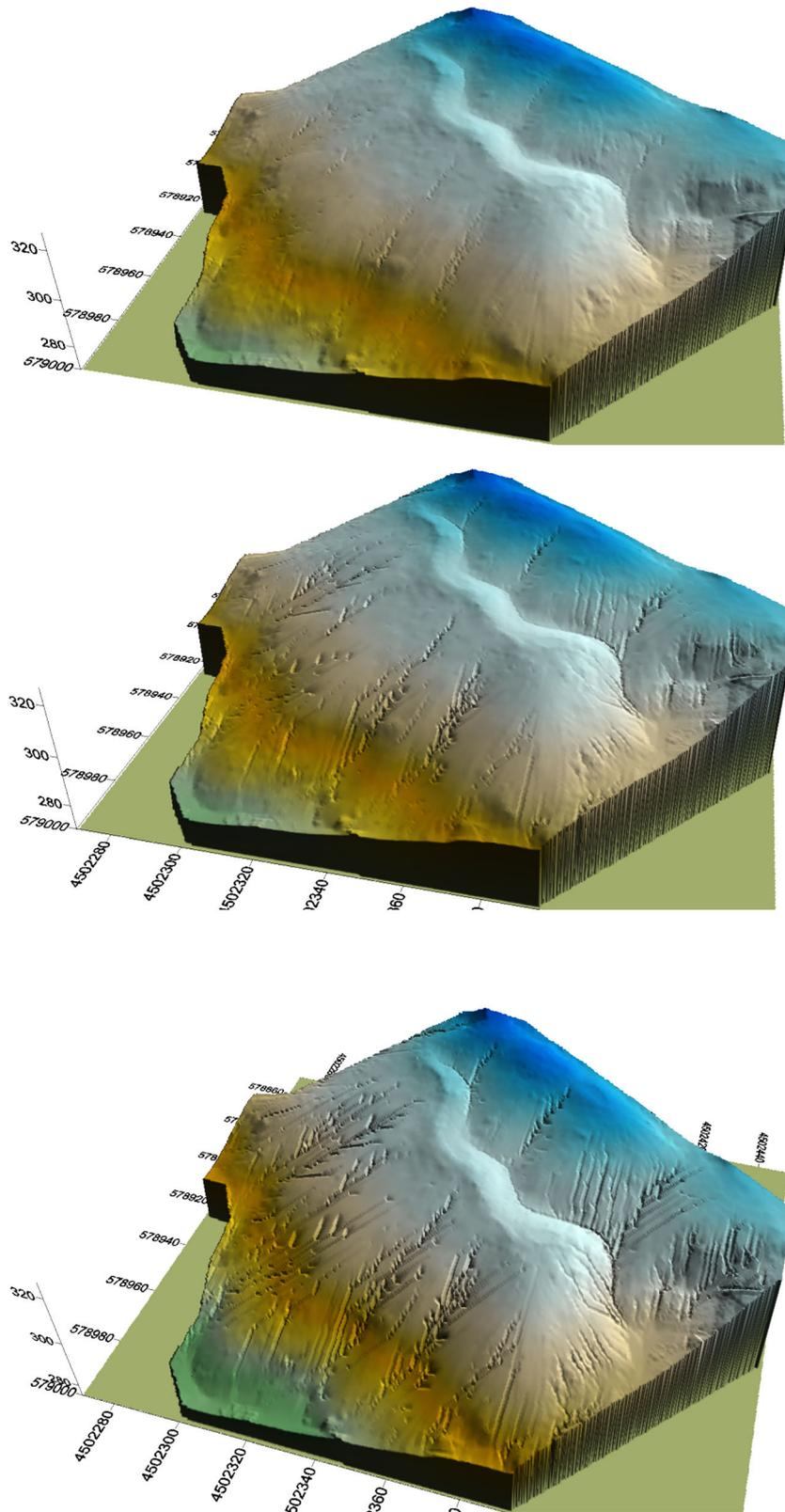
**FIGURE 11** West waste rock dump initial landscape at 10 (top), 50 (middle) and 100 years (bottom) using high erosion parameters. All dimensions are metres. [Color figure can be viewed at [wileyonlinelibrary.com](http://wileyonlinelibrary.com)]
