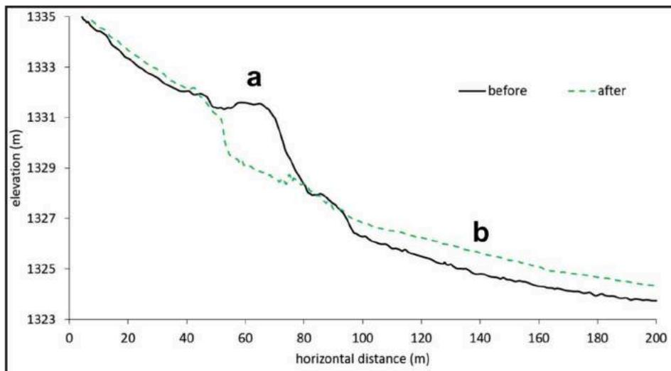
Fig. 6. Profile of gully erosion (a) and deposition (b) in the unpaved road and ditch (see Fig. 4).
