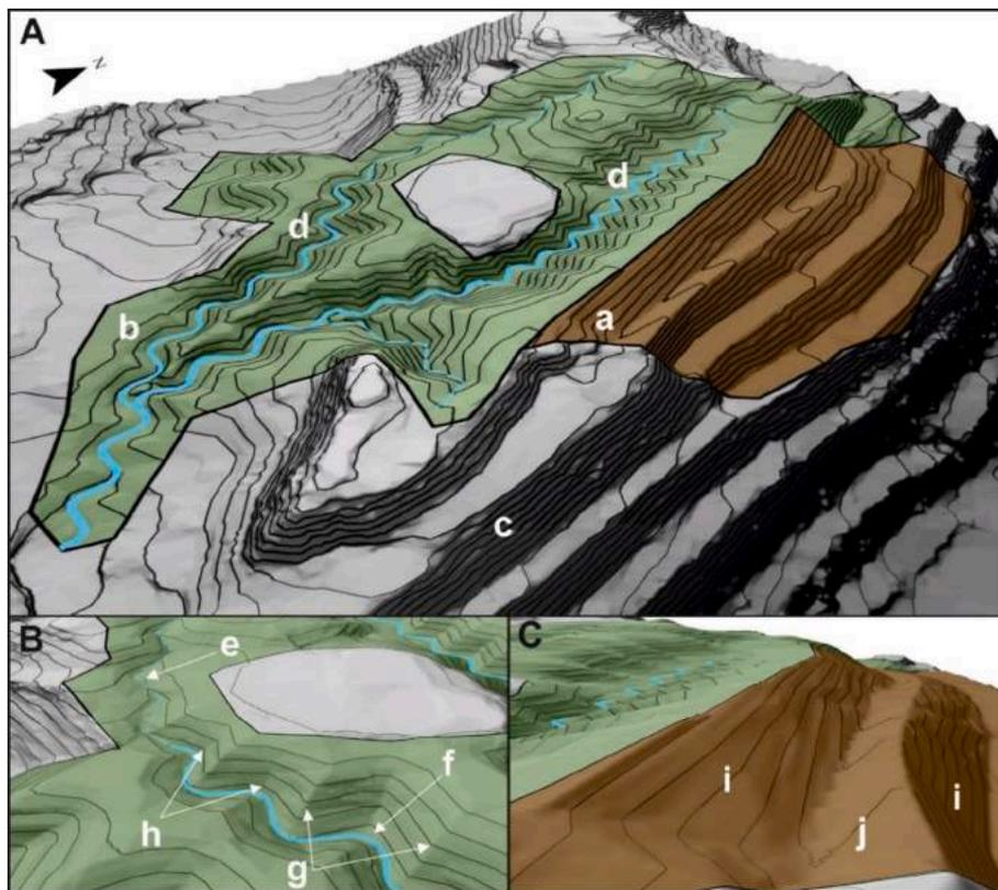
**Fig. 8.** A series of 3D views of the geomorphic and terrace rehabilitation design for “β2” waste dump in the Nuria mine: general (A) and details (B and C). (a) reclaimed area in terraces; (b) geomorphic rehabilitation; (c) original surrounding topography; (d) main channels with zig-zag (e) and meander (f) patterns; (g) convex-concave sub-ridges; (h) concave swales; (i) outslope; (j) berm with inverted gradient.
