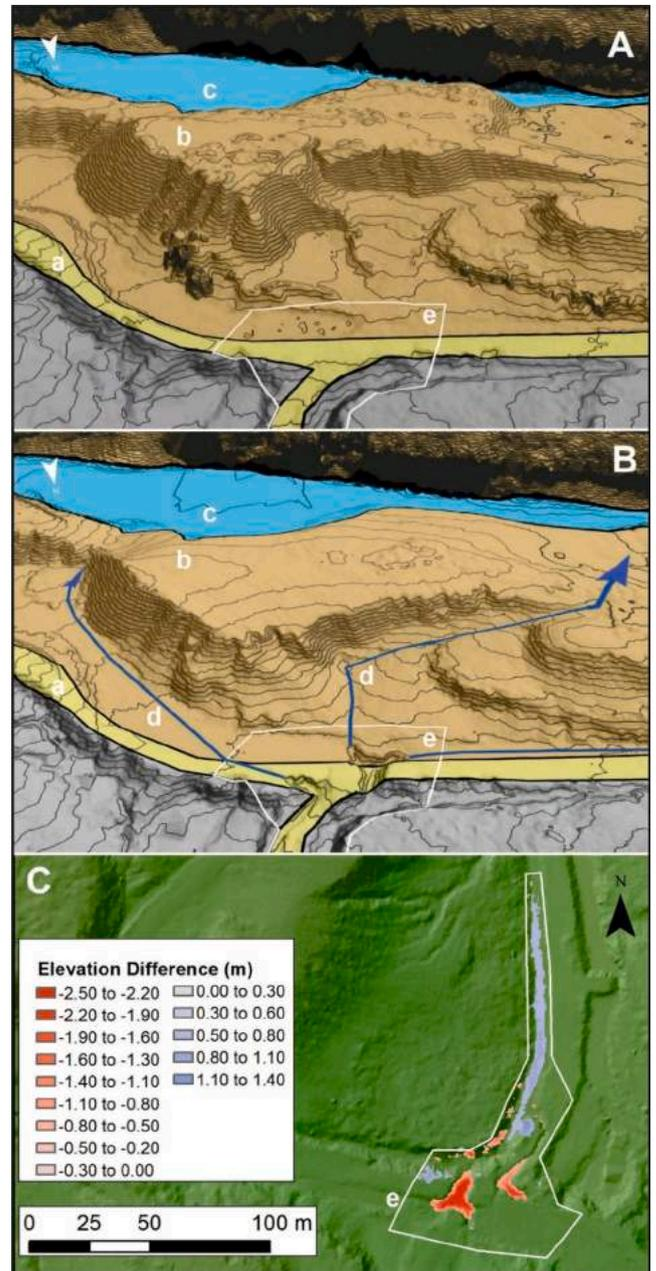
**Fig. 5.** Topography before (A, 2010) and after (B, 2018) gully development. (C) DoD showing (a) unpaved road; (b) area between the ponds and the unpaved road; (c) pond; (d) likely evolution of gully erosion; (e) polygon used to calculate the DoD in the gullied area. The arrows in B show the direction of knickpoint migration.
