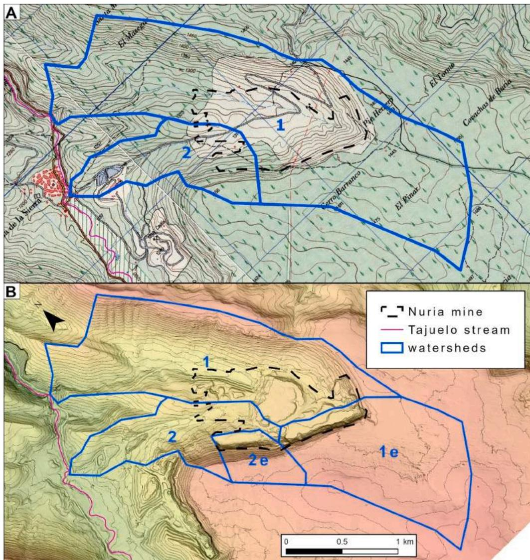
**Fig. 2.** Catchment evolution in the Nuria mine: (A) 1984, before mining; (B) 2018, after mining; (1, 2) natural catchments; (1e, 2e) mining-modified endorheic catchments with ponds at the highwall toe. A 25,000 map and a DEM and contours are the background for each date.
