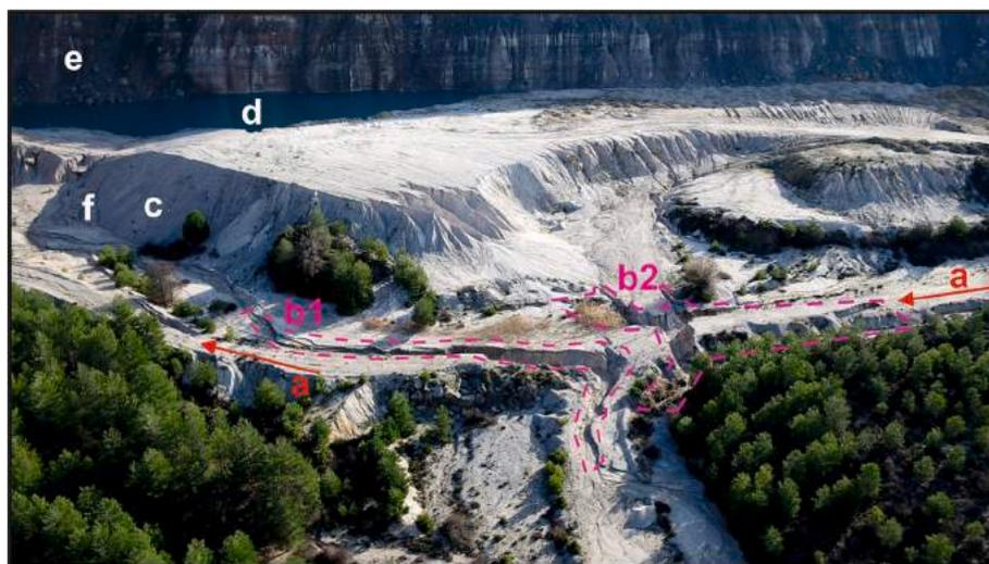
**Fig. 9.** Oblique photo of the main active gully erosion in the Nuria mine threatening an upstream pond (photographed on 26.03.2020). Road (a); left (b1) and right (b2) headcutting gully erosion; earth—sand—dam (c) enclosing the pond (d); highwall (e); weakest area in the earth—sand—dam (f). Photo by DGDRONE (2020).
