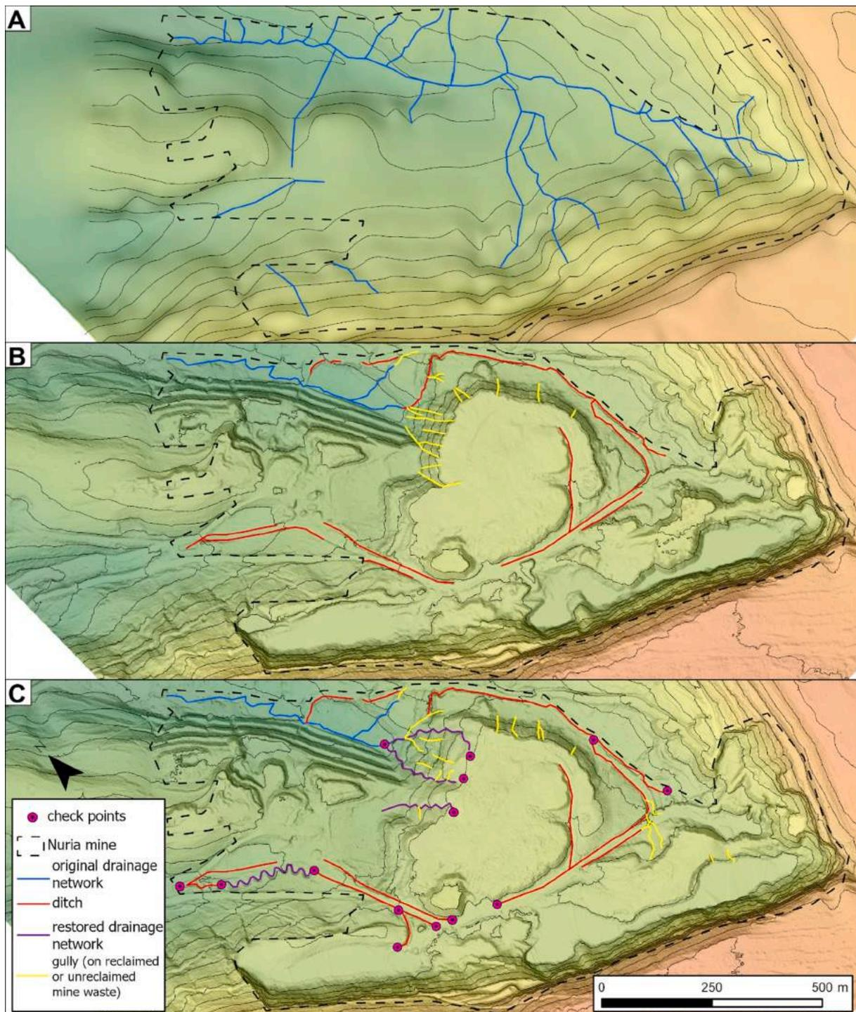
Fig. 3. Temporal change in drainage network and type of drainage lines around the Nuria mine: (A) 1984, (B) 2010 and (C) 2018. A DEM and contours are the background for each map.
