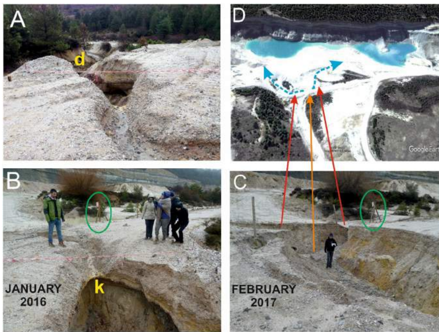
Fig. 5. Accelerated headcut gully erosion within the abandoned kaolin Nuria mine, in Central Spain, involving high flash flood risk hazard. A) Downstream view of the head of a gully, cutting an existing haul road, as a consequence of the drainage network re-development from the ditch (d) of the haul road. B) Position of the knickpoint (k) in January 2016. This photo shows the same location of photo A, but in opposite direction. C) Same location that B in February 2017; the knickpoint has migrated upstream about 20 m in length and about 2 m in depth in 13 months, cutting completely the haul road. Note the fence post within the green ellipse for comparison. D) At the location of the person in photo C, the gully has developed two branches, which are head cutting towards a large pond located at the foot of the highwall of the former mine (blue arrows). If the headcut reaches the pond, a flash flood will occur, risking a village, a main road and a natural park located downstream of this location. The mine is abandoned (with no rehabilitation). But even a proper rehabilitation, with successful soil and vegetation recovery, but lacking to understand this process, would have likely led to the same results. (For interpretation of the references to colour in this figure legend, the reader is referred to the web version of this article.)
