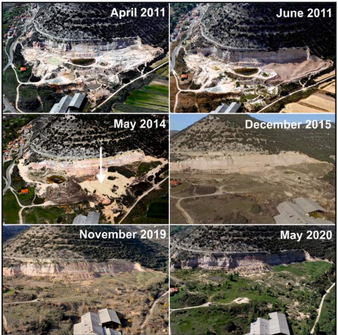
**Fig. 7.** Comparison of oblique aerial photos of the Somolinos quarry from April 2011 (before restoration) to May 2020. Notice the 1-ha surface restored in June 2011. At the May 2014 photo, the lighter colours (white arrow) are the central area left without manure amendment. Photos by Paisajes Españoles (years 2011 and 2014), David Gutiérrez (DGDRONE, years 2015 and 2020) and Javier Meleró (year 2019).
