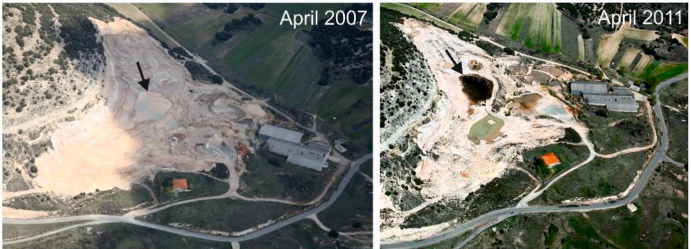
Fig. 3. The 2007 image shows the quarry closure and stabilization works, regrading platforms and sediment ponds construction (the black arrow points to the main one, which is the one visible at Fig. 2F). As it can be seen in the 2011 image, four years later, the surface had not recovered any soils or vegetation. Photos by Paisajes Españoles.
