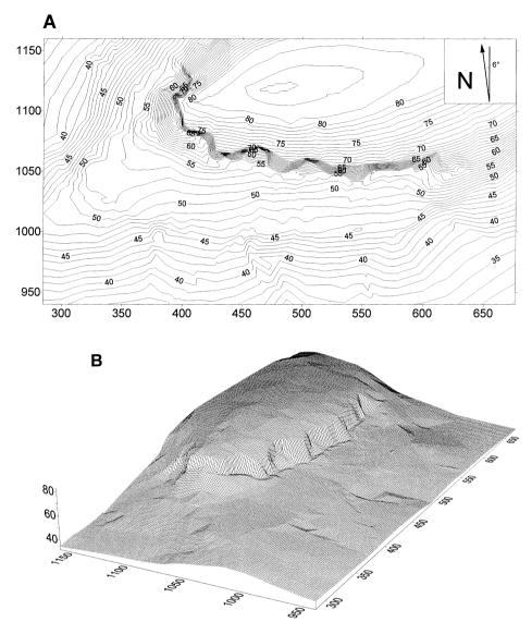
Fig. 6. Projected situation following rehabilitation. A: final contour map. B: block diagram seen from the SW (SURFER 5.1 program). Distances in metres.
