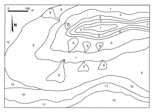
Fig. 3. Map of the geomorphological units in the area around the 'La Revilla' quarry. The working of this quarry affected units 5, 6, 7, 8 and 9. The description and features of each unit are supplied in Table 1.
