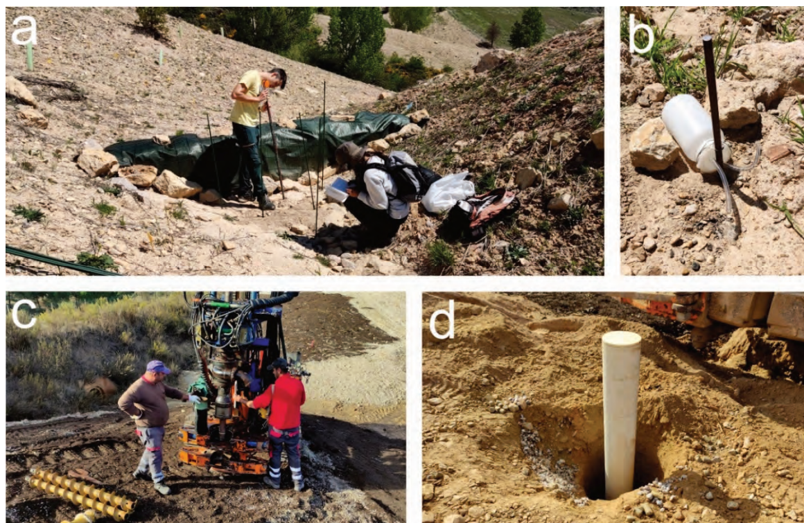
Figure 12 Monitoring procedures deployed to measure and quantify the improvement of water quality from the restored mined areas within LIFE RIBERMINE. (a) Check dams to measure total sediment yield (Peñalén, Spain); (b) Syphon bottles to sample SSC (Peñalén, Spain); (c) Installation of piezometer at Lousal (Portugal) to monitor water table and to take water samples; (d) Detail
