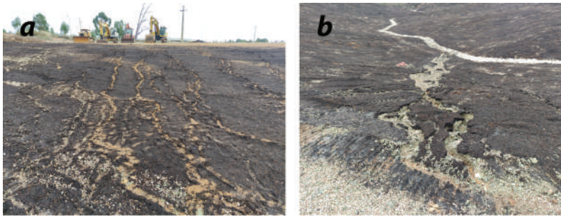
Figure 8. Rilling processes in the reclaimed area near the encapsulated pyrite deposit; (a) Small rills of 5–10 cm width and 2 cm depth; (b) Rills of 20–30 cm width and 10–20 cm depth.
